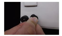
③ The AC switching lever can be seen through the hole uncovered when the cap is removed. By using long-nose pliers and so on, switch to the voltage of the power source being used.
