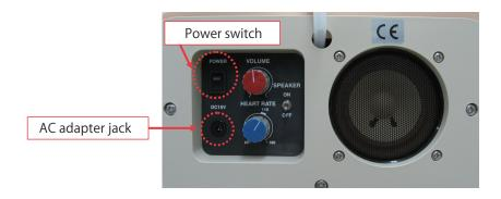
2) Adjust the fetal heartbeat volume with the VOLUME dial on the panel, and the speed of the fetal heartbeat with the HEART RATE dial. The SPEAKER switch is used to switch emission of the fetal heartbeat sound to an external speaker.
