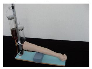
11. Open the pinchcock to allow the simulated blood to circulate.
