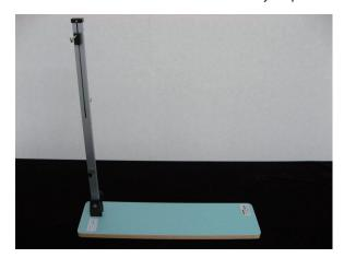
4. Set the arm support rod on the stand hook. Align the elliptical hole with the hook and set the rod in. The arm support rod will not come off when the fist is lowered onto the base.
